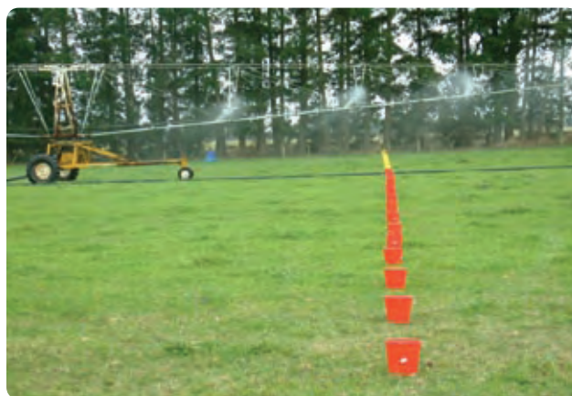
Figure 7. Measuring distribution uniformity of a travelling boom irrigator
